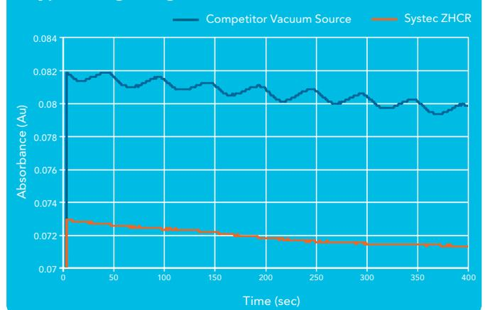
Fluctuations in detector baseline of a single-speed pump compared to the patented technology of the Systemc ZHCR vacuum pump.\* UV detector baseline fluctuations are minimal when compared to traditional stop and start vacuum sources.
