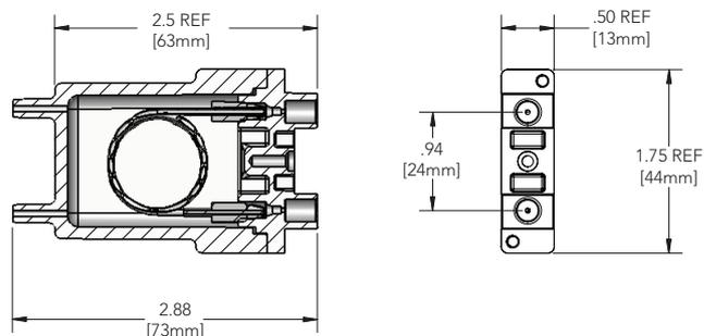
Dissolved gases are actively removed from a flowing liquid stream by vacuum via the Systec AF membrane.
