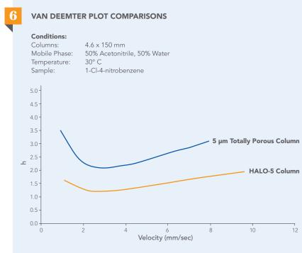
This comparison of van Deemter plots for HALO-5 and a totally porous 5 micron particle demonstrates the extraordinary low reduced plate height that is obtained from HALO-5 columns. The unusually narrow particle size distribution of the HALO-5 Fused-Core particles facilitate the packing of columns with efficiencies (theoretical plates) that are significantly larger than what would be expected from the size of the particles.
