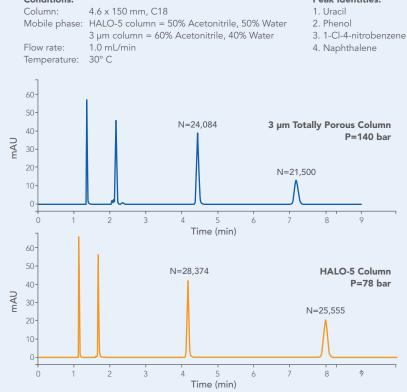
HALO-5 columns generate over 17% more plates than an HPLC column of the same dimension packed with 3  $\mu m$  totally porous particles, but generates less than 60% of the back pressure.
