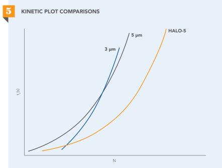
Kinetics plots are used to compare columns packed with different particles and particle sizes. This Kinetic plot compares columns of various lengths packed with HALO-5, 5 micron totally porous and 3 micron totally porous particles and shows that HALO-5 columns provide more column plates (N) for a given analysis time ( $t_o$ ) than columns packed with totally porous 5 and 3 micron particles.
