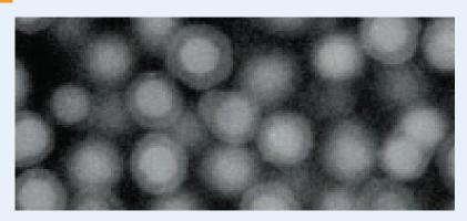
This SEM photograph of "sliced" Fused-Core particles clearly shows the structure; a solid core surrounded by a porous "halo".
